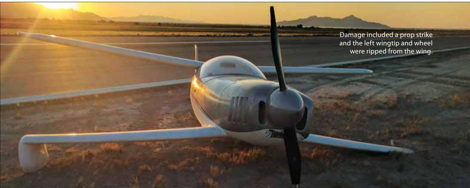
Damage included a prop strike and the left wingtip and wheel were ripped from the wing.
