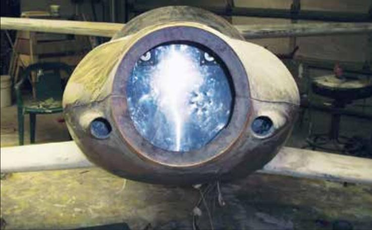
Original Q2 cowl lengthened with enlarged spinner. Small intakes were fabricated around soda cans.
