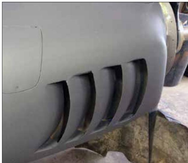
What a difference the primer makes. Access panel moulded in place assures a good fit.
