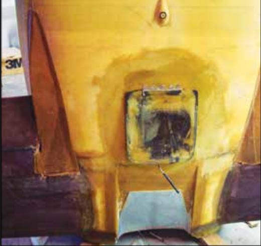
Fitting and trimming the fairings. They will later to be glued in place.
