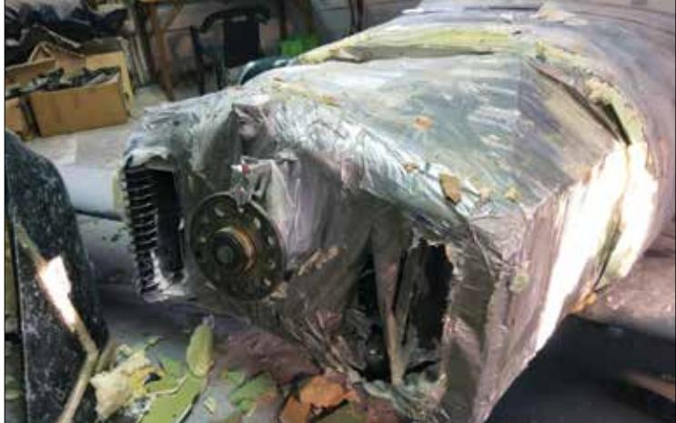
Engine wrapped with plastic and duct tape for a new plug and mold.
