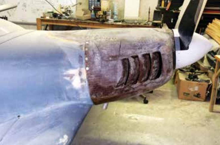
Fitting the cowl after trimming and sanding.
