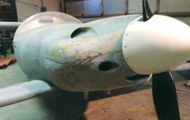
Final iteration of the original cowl. Middle intake sanded off, then lensed for a landing light. New radiator cooling intake just beneath the spinner.
