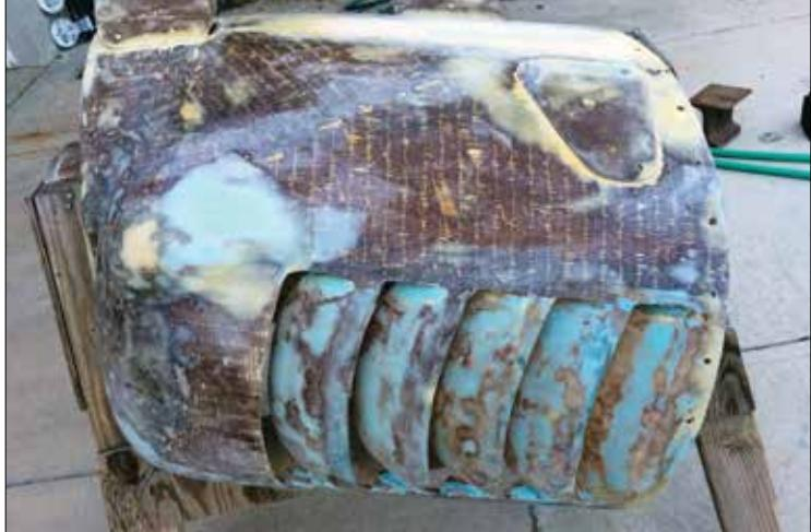
The final cowling, sanded, filled and ready for primer.
