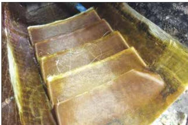
Glass curing over clay louvers in the mold.
