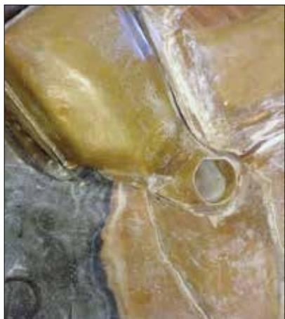
Complicated induction filter mount and plumbing moulded over clay.
