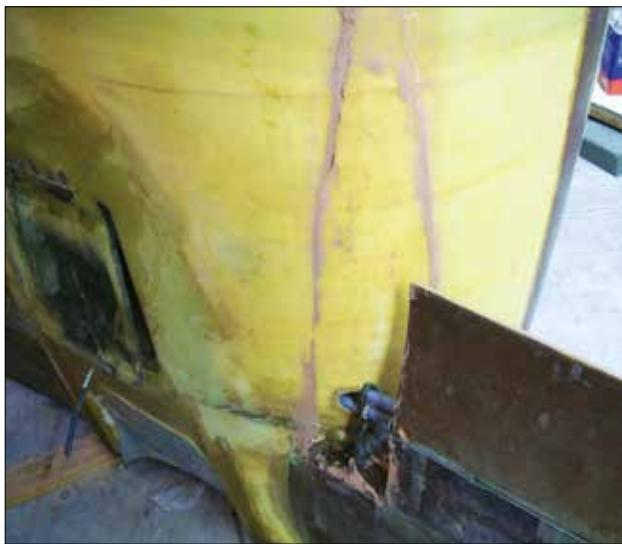
Clay residue still remains on fuselage after forming wing root fairings. It's easily cleaned up with MEK and a wire brush.
