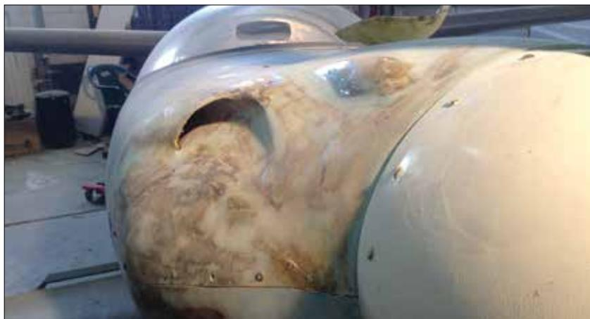
Intake for the oil cooler and starter bump was formed over clay, then glued in place.
